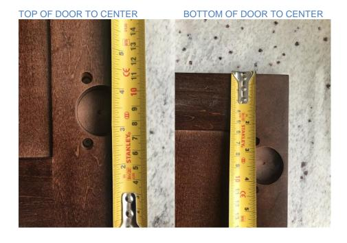
MEASURE PANELS REQUIRED WIDTH 11 7/8 OR 300MM HEIGHT 30 7/8 OR 784MM
